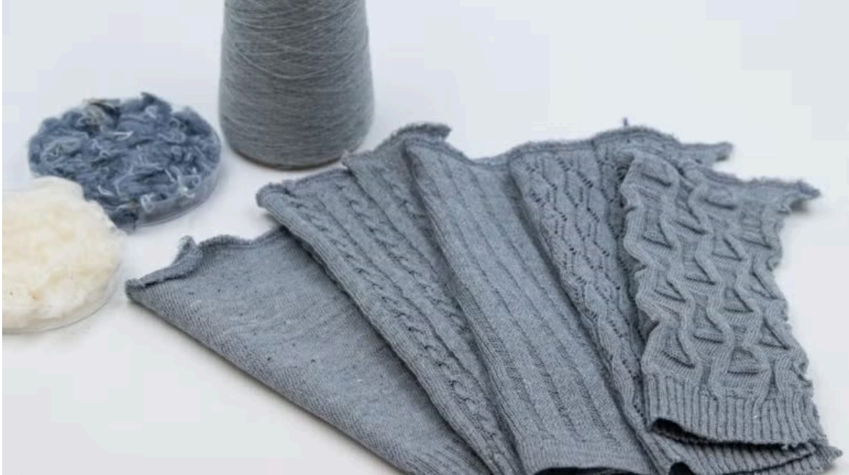
Knitted fabrics using yarn made of mechanically opened cotton fibres from post-consumer denim. Credit: Susanna Raiskio at VTT.
